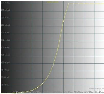
*PQ 300 cd/m<sup>2</sup> clipping after hardware calibration*
